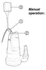
To ensure that the pump draws the water out, the water to be drained must be at least 45 mm deep.
